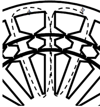
Figure 3: Operating principles of DSSPM motor
