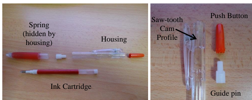
Figure 5 Components of Retractable Pen
