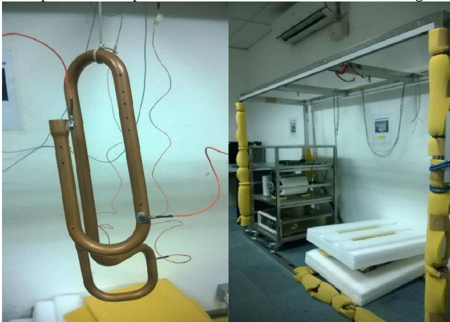
Figure 5. Experiment set-up of suction tube (left) and insulated test rig (right)
