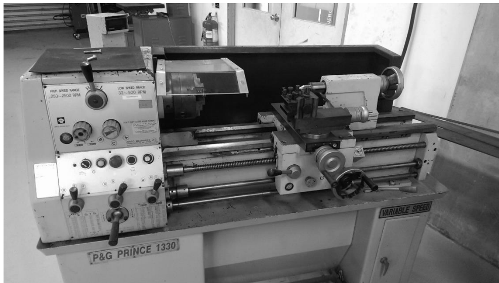
Figure 7. Lathe machine provides rotation speed up to 2500 RPM.
