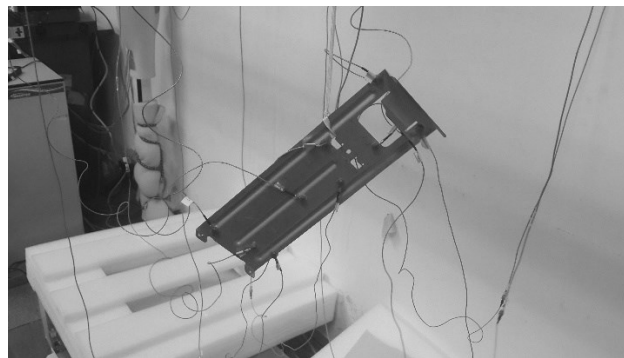
Figure 2.3 Sensor Placement and Hanging Method
