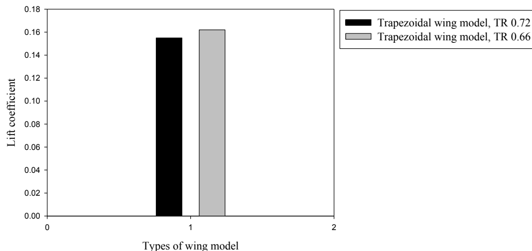
Figure 10: Lift Coefficient for various taper ratios Trapezoidal wing models at 140000 Reynolds number
