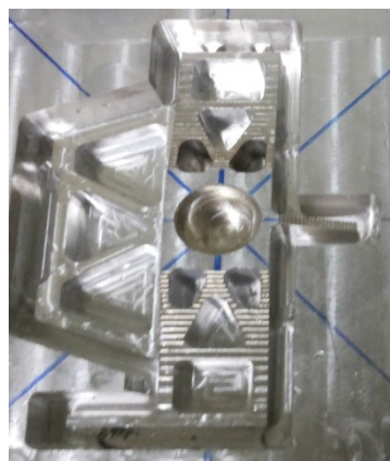
Figure 13. Manufactured upright using CNC milling machine
