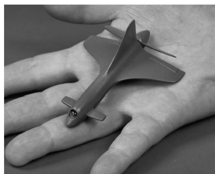
Figure 3. Example of micro-air vehicle with 7.3 cm wingspan [9]
