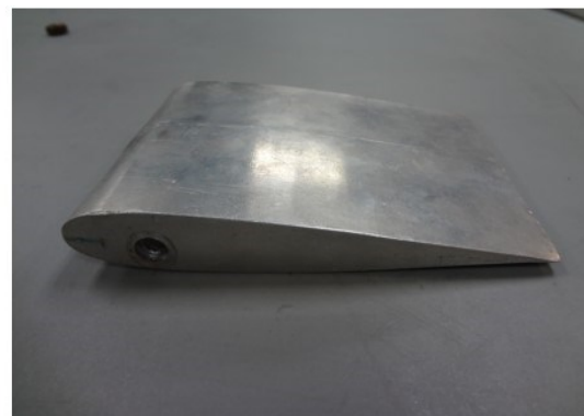
Figure 5. Aerodynamic Centre of Airfoil (Left) and Steel NACA 0012 Airfoil (Right)
