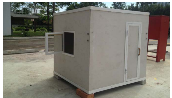
Fig 2 The Fabricated Room of 1x1x1 m and 2mm Wall Thickness
