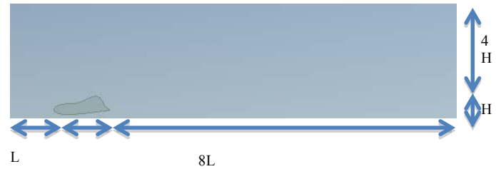
Fig 1. Computational Domain for CFD Simulation Setup (Front View)
