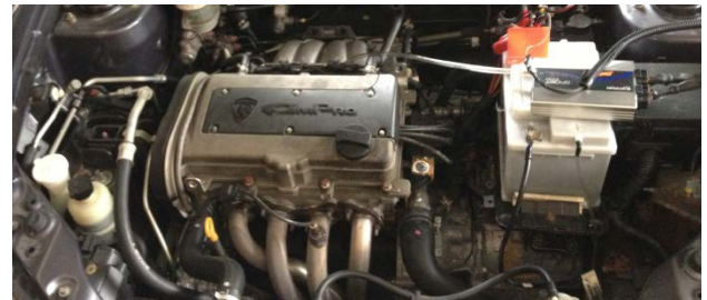
Figure 1: Campro S4PH Engine
