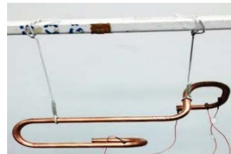
Fig. 1 The “free-free” boundary condition set-up for EMA
