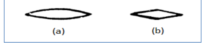
Fig. 2 The investigated airfoils (a) biconvex (b) double wedge
