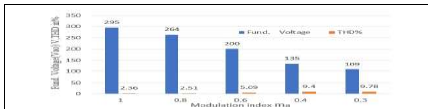
Fig.15 Variation of THD and fundamental output voltage with respect to modulation index m_a
