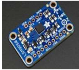
Fig. 3. Accelerometer / Magnetometer / Gyroscope Temp 9-DOF Breakout Board LSM9DS0 Adafruit
